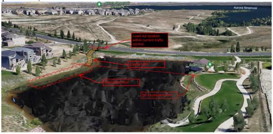
RCD pumped water out of the pond for 4 weeks to get it down to a working level so they could begin dredging. RCD was required to capture the sediment through 2 settlement tanks and a silt bag at the outlet pipe before the water was discharged into the storm system, and set up and maintain appropriate BMP measures including street sweeping. This dewatering was supposed to be done before RCD started and was not part of the original scope.
